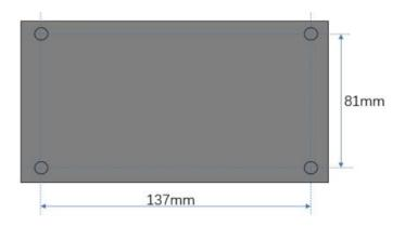
步骤2. 使用钻孔设备在面板上已标记的安装孔位置钻孔。Use drilling equipment to drill holes in marked mounting positions on the panel.
