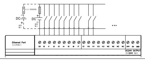
◆ 因为公共端 CO/C1/C2 彼此独立,使用相同输入类型时,请使用短接线将公共端连接。As the common terminals CO/C1/C2 are independent of each other, when using the same type of input, please connect the common terminals using short wires.
